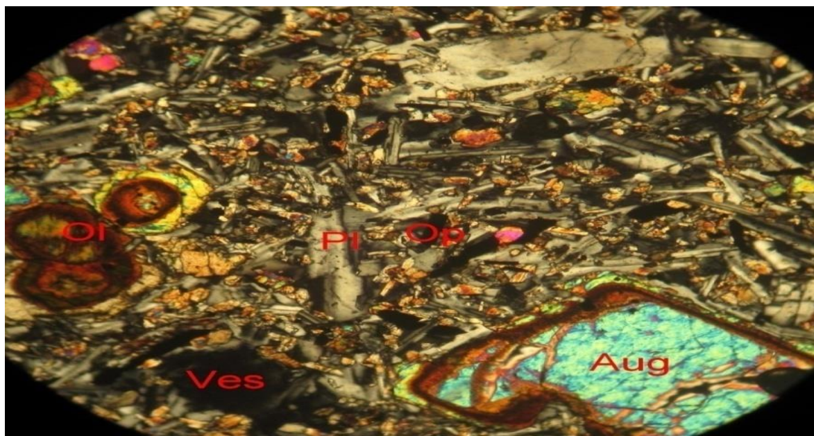
Figure 2: Photomicrograph of MIA, XPL showing 35% of Hortonolite and 10% of Ferro-augite rounded by rims (pigeonite?), 35% of Andesine and 25% of Ulvospinel
