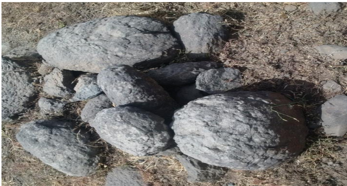
Figure 3: Alkaline Olivine basalt at Miango Volcanic Field with total alkaline content greater than 3% and modal olivine greater than 5%.
